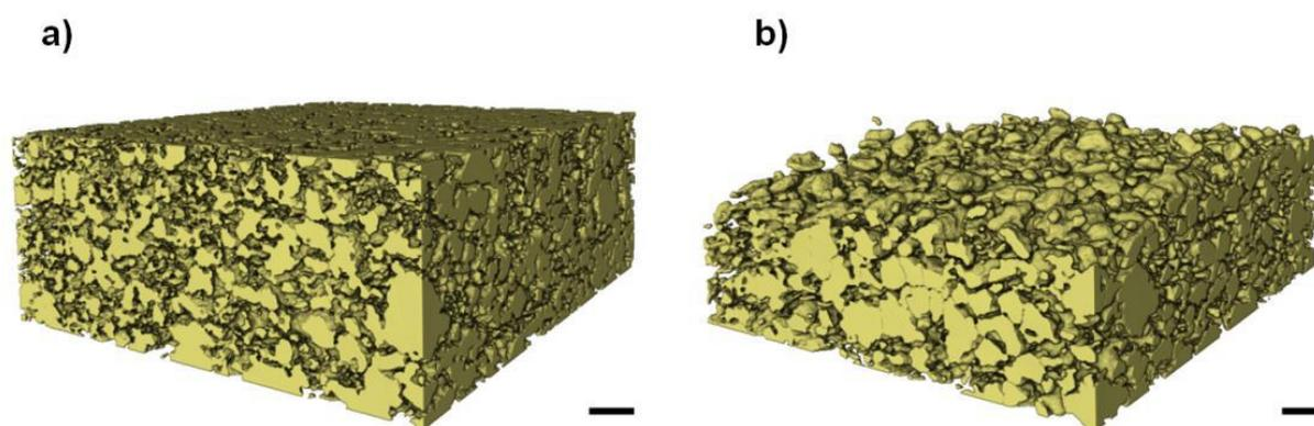
Figure 1. Volume rendering of the sulfur phase for (a) the uncycled cathode and (b) the cathode after 10 cycles. Scale bar represents 50  $\mu\text{m}$ .
