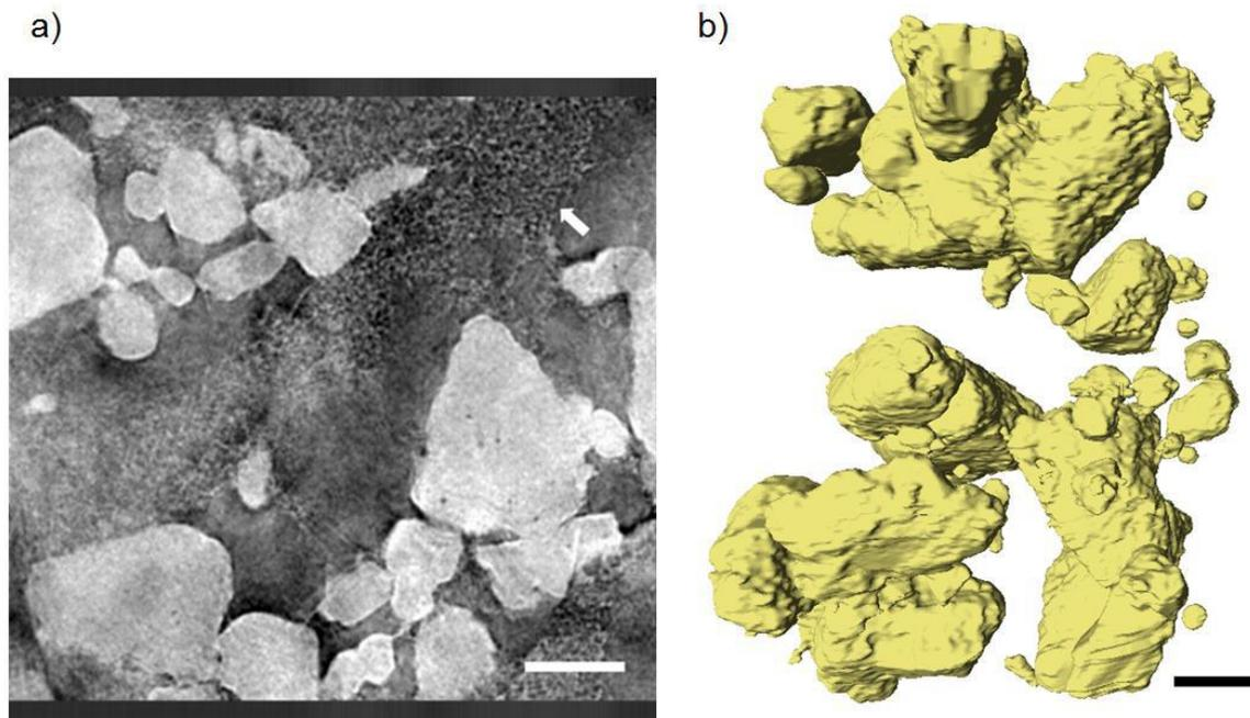
Figure 2. left (a) X-ray Zernike phase contrast nano-CT on S-composite used, carbon binder domain indicated by the white arrow; right (b) volume rendering of segmented sulfur particles. Scale bars represent 10  $\mu\text{m}$ .
