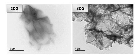
The synthesis of 3D graphenes is carried out from graphitic oxide (GO), derivative of graphite. GO is prepared by the modified Hummers' method, and subsequently, by means of a reduction step, 3DG are obtained using a hydrothermal treatment with determined conditions of pressure and temperature. The properties of 3DG are improved by doping with nitrogen, thanks to the use of urea.<sup>1</sup>
