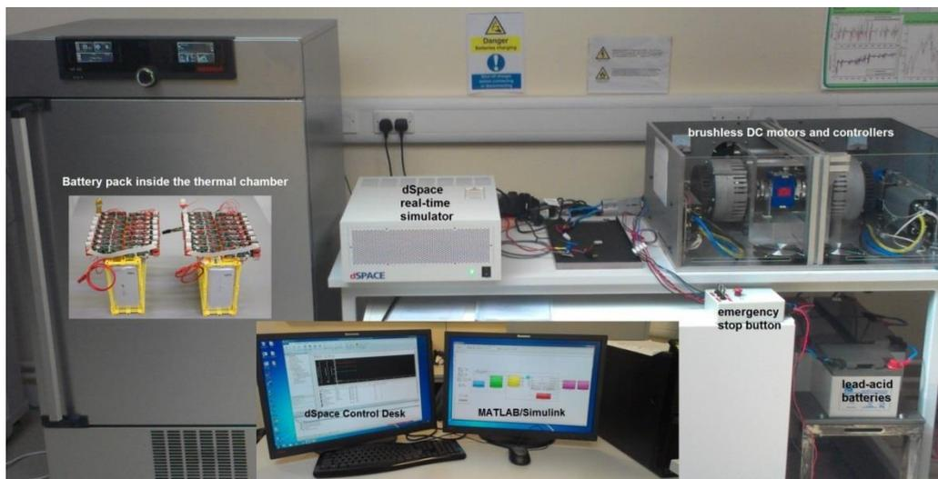
Figure 1: hardware-in-the-loop (HIL) test rig for test and development of EV battery management algorithms
