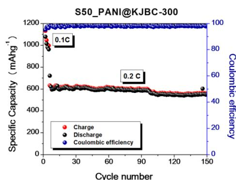
Capacity vs. cycle number of Li/S cell with PANi wrapped KJBC/S composite cathode in DME:DIOX 1:1 (v/v) 1M LiTFSI 0.25M LiNO<sub>3</sub>. Sulphur loading 55%, PANi loading: 35%..
