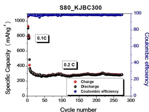
Capacity vs. cycle number of Li/S cell with KJBC/S composite cathode in DME:DIOX 1:1 (v/v) 1M LiTFSI 0.25M LiNO<sub>3</sub>. Sulphur loading 80%
