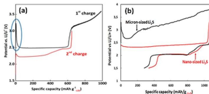
**Figure 1:** (a) Typical voltage profiles of two first charges of a  $\text{Li}_2\text{S}$ -based cell [1] and (b) comparison of voltage profiles between micro and nano-sized  $\text{Li}_2\text{S}$  particles-based cell.
