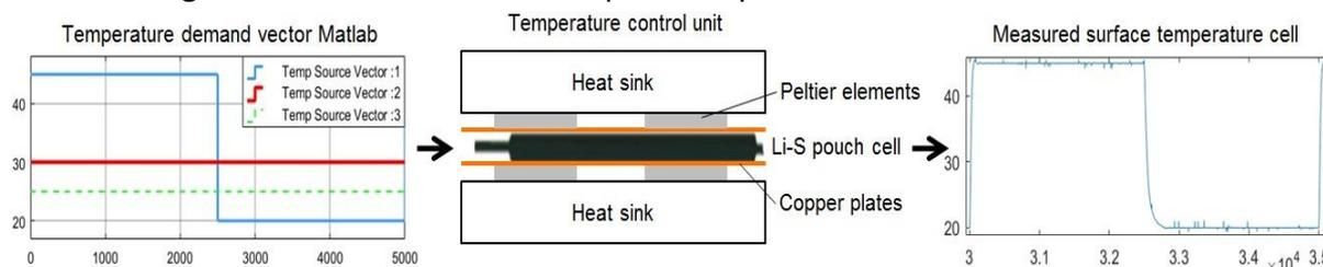
The finished poster will incorporate details of the test rig approach as well as an initial cell discharge test result for a current pulse discharge in combination with a mixed temperature profile.
